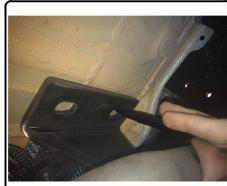
4. Lower the hitch and use a drill and 5/16" drill bit to drill (5) holes located at the marked areas from step 3. Then use 9/16" drill bit to open up the holes to the final size.
