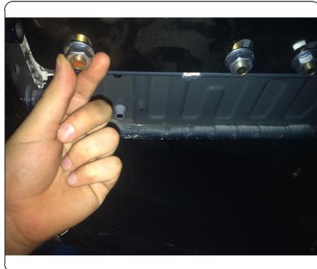
5. Use an 11/16" socket and torque all 7/16" hardware to 70 ft-lbs. Raise exhaust back into position and reinstall rubber isolators removed in Step 1.
