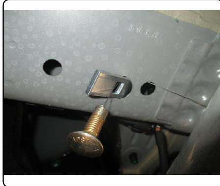
4. Gently pull fascia down and raise hitch into position guiding fishwires through mounting holes. NOTE: Hardware may need to be temporarily pushed into frame to position hitch over bumper beam studs. Remove fishwires & loosely secure 7/16 nuts. Secure existing M10 nuts onto bumper beam studs.
