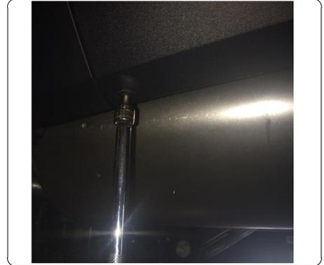
2. Fishwire (3) CM-SP2 spacers and (3) 7/16" carriage bolts through access hole and out mounting holes on each side of vehicle. Raise hitch into position and secure with (3) 7/16" flange nuts on each side. (As shown in the Fishwire Technique Diagram)
