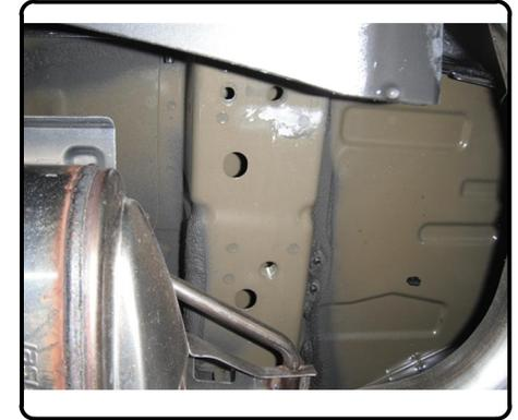
3. Raise hitch into position between exhaust tip(s) and attach to vehicle using the supplied 12mm bolts and washers.
