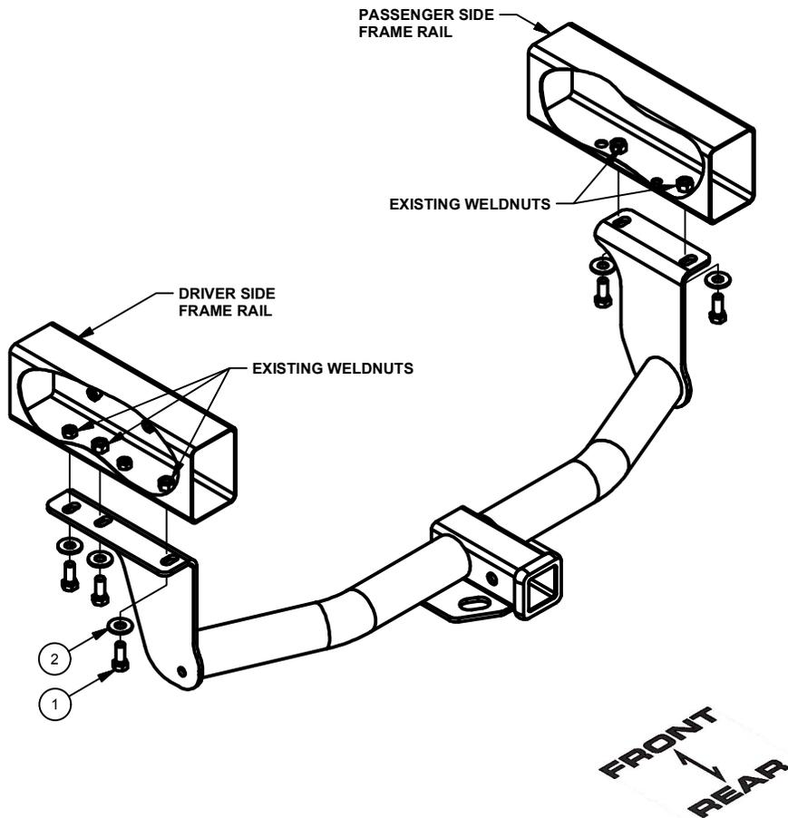
1. If present, remove the (4) bolts holding the tie down bracket onto the vehicle and return to the owner.
