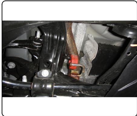
2. Remove the (1) fastener securing the heat shield to the bottom of the driver side frame rail. Trim the portion of the heat shield covering the mounting areas of the driver and passenger side frame rails, see trim diagram. After trimming re-attach the heat shield to the bottom of the driver side.
