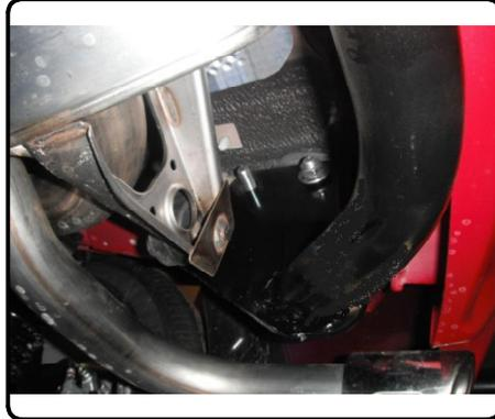
4. Align the bottom tabs of the hitch with the weldnuts in the frame rails and secure with M10-1.25 x 25mm bolts and 3/8" conical toothed washers.
