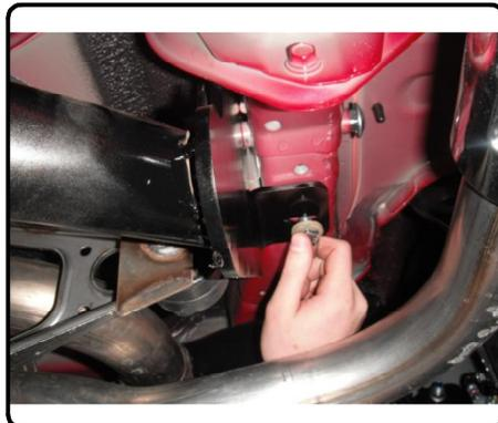
5. Torque all 10mm hardware to 48 ft-lbs. Torque all 1/2" hardware to 110 ft-lbs.
