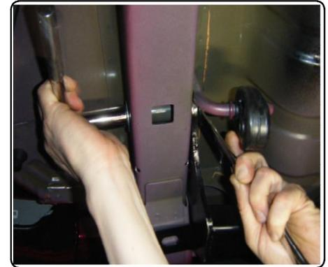
8. Reinstall heat shield, fasteners, and exhaust.
