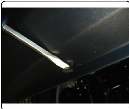
2. Lower exhaust by removing (3) rubber isolators. See RUBBER ISOLATOR REMOVAL DIAGRAM on page 2. (**Note:** Support exhaust to avoid possible damage.)
