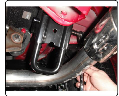
2. Insert 1/2-13 x 4 1/2" carriage bolts and CM-12048-SP spacers through the existing holes in the side of the frame rails. After bolts are inserted push them back so the end is flush with the inside of the frame rails.
