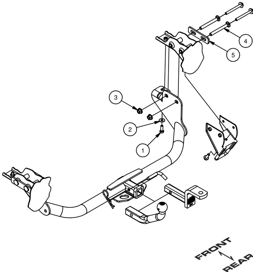
1. Remove (3) bolts and tow loop from the passenger side frame rail. Return bolts and tow loop to owner
