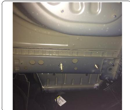
5. Torque 7/16" hardware to 70 ft-lbs. Reinstall trimmed underbody panel removed in Step 3. Raise exhaust back into position and reinstall rubber isolators as removed in Step 1.
