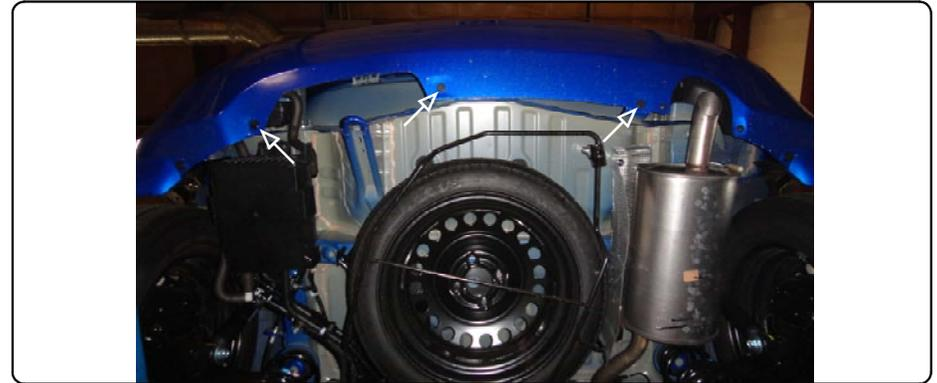
2. Mark and trim rear fascia. **Note:** Dimensions are approximate, confirm fit prior to trimming. See Fascia Trim Diagram
