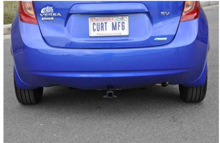
**11378****NISSAN VERSA NOTE****10/30/2013****GROSS LOAD CAPACITY WHEN USED AS A WEIGHT CARRYING HITCH: 2,000 LBS. TRAILER WEIGHT & 200 LBS. TONGUE WEIGHT.**
