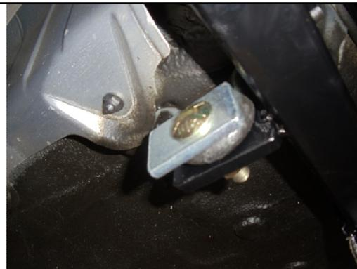
4. Raise hitch into position and loosely attach 7/16" hex flange nuts to carriage bolts.
