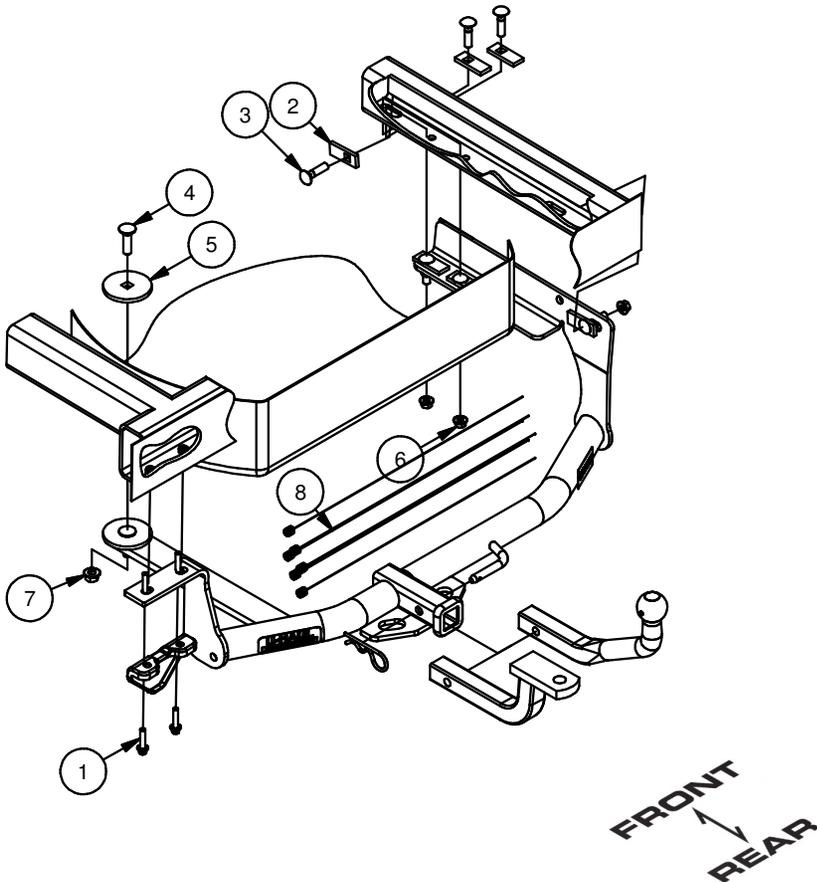
1. Lower the passenger side underbody panel by removing (3) torx head screws and (2) hex nuts. (Save fasteners for use in Step 10.)
