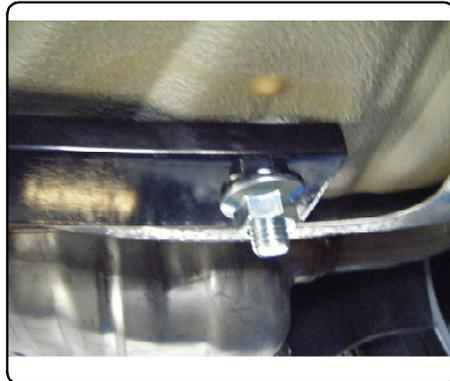
9. Torque all M8 hardware to 17 ft-lbs., all 7/16" hardware to 70 ft-lbs. and all 1/2" hardware to 110 ft-lbs. Trim rear underbody panel to clear the passenger side plate as shown in the Underbody Panel Trim Diagram. Reinstall the underbody panel using the torx head screws and hex nuts removed in Step 1.
