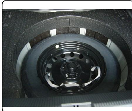
5. Remove the middle plug on the driver side of the spare tire well. Return plug to vehicle owner.
