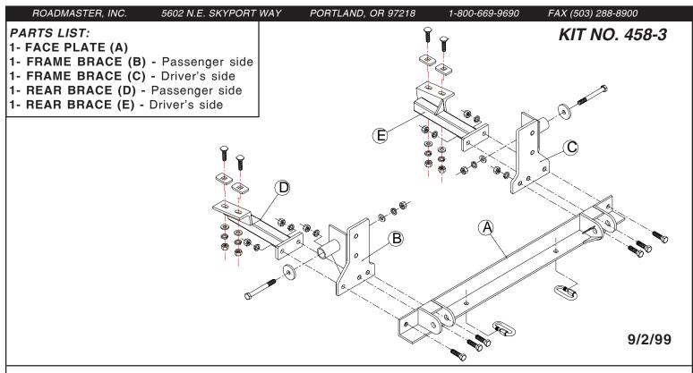
**IMPORTANT:** All brackets **must** be assembled with all the bolts left loose for final adjustment & positioning (before tightening) unless otherwise instructed. All bolts **must** be torqued for proper strength. If more than one bolt is used per fastening point, the diagram may only show one.
