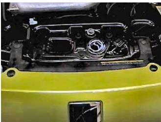
1. Remove the two push pins from top edge of fascia.
