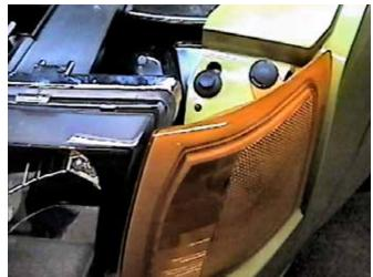
2. Remove the metric bolt and one push pin from blinker assembly with the 10MM socket, both sides, pull forward, unplug electrical and set aside.
