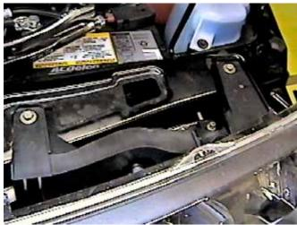
Using the 6MM socket, remove two metric bolts from headlight assemblies, pull forward, unplug electrical connections and set aside, on both sides.
