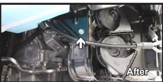
18. To reattach the horn, use the existing hole in the frame webbing on the passenger's side and the existing hole on the horn bracket, insert a 1/4"-20 x 3/4" hex bolt with a 1/4" lock washer and 1/4"-20 nut. Reattach all electrical connections.
