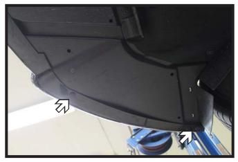
3. On the underside of the fascia remove the two (2) pushpins from the outer edge. Repeat this on the other side of the vehicle.
