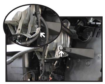
11. On the driver's side, use a 8MM socket to remove the bolt from the frame webbing. Once the bolt is removed, bend the webbing outward with a pair of large vice grips far enough to fit the baseplate on top of it.
