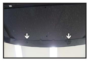
4. On the underside of the fascia remove the two (2) pushpins from the front outer edge.
