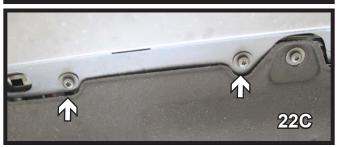
22. **Optional:** To install a breakaway switch, you must remove the belly pan with a T30 Torx. Remove the two (2) screws from in front of both the driver's and passenger's side tires (22A) then follow the pan toward the middle of the vehicle removing the three (3) specified bolts (22B and 22C).
