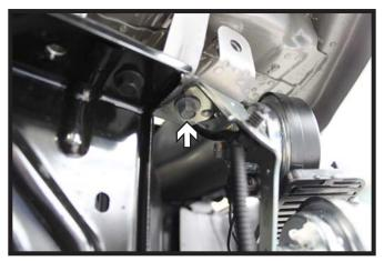
7. Using a 10MM socket, remove the bolt from the passenger's side horn bracket. Disconnect and set horn bracket aside.
