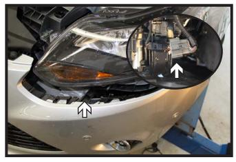
On the driver's side, locate the running lights main electrical cord and disconnect. Under both headlights release the tabs from the body and carefully remove the fascia.
