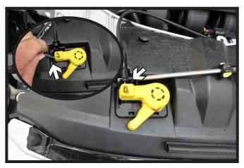
5. Using a flat screwdriver, pry the black hood latch cable out of the black mounting bracket (white arrow). Then rotate the wire left to release it.
