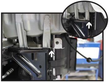
On the passenger's side only, use a reciprocating saw to remove the washer reservoir bracket and horn front bracket.
