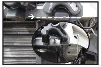
12. On the plastic bumper cover, using a utility knife, trim the lower outer edge flush with the bottom of the bumper. Repeat on the other side of the vehicle.
