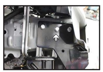
16. If necessary, drill a hole through any obstruction from frame webbing in the middle hole of the baseplate with a 13/32" drill bit. Insert a 3/8"-16 x 1-1/2" hex bolt and 3/8" lock washer with a 3/8"-16 nut plate. Do this on both sides.
