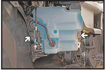
Using a 10MM socket, remove the two
