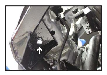
15. Using the baseplate as a template, drill a hole through the bottom of the frame webbing using a 13/32" drill bit. Do this on both sides of the vehicle. Insert a 3/8"-16 x 1-1/2" hex bolt with a 3/8" lock washer and 3/8"-16 nut plate through the hole on the bottom of the baseplate. Make sure baseplate is level, then tighten. Do this to both of the bottom holes FIRST, then tighten the two (2) top bolts on each side (14).
