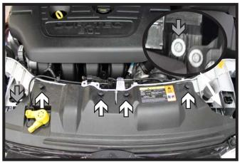
1. From the top of the fascia, using a T30 Torx, remove the inner-most bolt from each side (gray arrow). Remove the four (4) push pins (white arrows).
