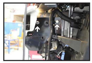
14. On the driver's side, slide the baseplate on top of the bracket we bent down earlier until the top back hole is aligned with the top back existing hole on the frame webbing. Insert a 3/8"-16 x 1-1/2" hex bolt and 3/8" lock washer with a 3/8"-16 nut plate. Also secure the top front hole the same way. **DO NOT** tighten bolts all the way, wait until directed to do so. Do this on both sides of the vehicle.
