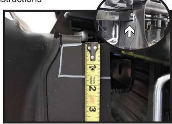
21. To reattach the intake cover, use a utility knife to cut from the back upper corner of the side wall a 2 1/2" x 1 1/2" rectangle from each side of the cover. Reinstall using the two (2) T30 Torx bolts. NOTE: If a breakaway will be installed, install the breakaway before installing cover. Be sure that bottom of the cover goes below the breakaway bracket.
