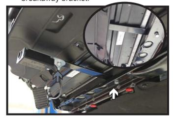
23. **Optional:** Using a 1/4"-20 x 1/2" hex bolt with a 1/4" lock washer, attach the breakaway bracket to an existing hole on the frame webbing, just slightly toward the passenger's side of the vehicle (white arrow). Attach the breakaway using a 1/4"-20 x 3/4" bolt, 1/4" spacer nut, and a 1/4"-20 nylon nut (gray arrow). Attach all electrical connections and reinstall the belly pan. NOTE:Breakaway should stick out the bottom of the fascia once reinstalled.
