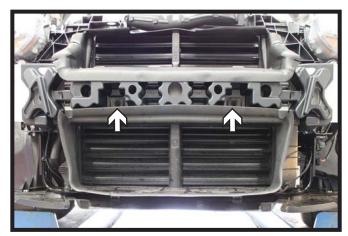
9. Using a T30 Torx, remove the flexible intake cover.
