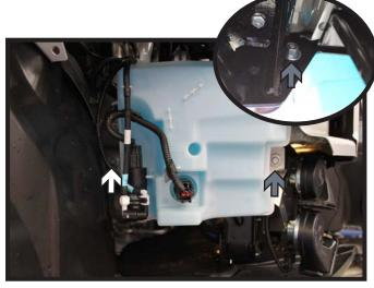
17. Reattach the washer reservoir on the passenger's side. Use the existing bolt in the back (white arrow). Then a 3/8"-16 x 1" hex bolt with a 3/8" flat washer and a 3/8" hex nut in the front hole thru the baseplate (gray arrow).
