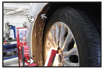
2. Using a T27 Torx, remove the two (2) screws from the driver's side front wheel well (white arrows). Remove the push pin from the driver's side front wheel well (gray arrow). Repeat this on the passenger's side.
