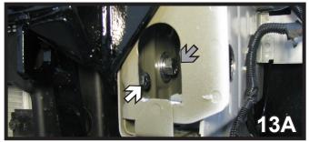
13. Using the baseplate as a template, insert 3/8-16x1" hex bolts with Loctite, 3/8" lock washers and 3/8" flat washers into the two outside holes and tighten down with a 3/8-16 hex flange whiz lock nuts (see white arrows). On the inside hole use a 1/2-13x1" hex bolt with Loctite, 1/2" lock washer and 1/2" flat washer tightened to a 1/2" wire nut inserted into the frame (see grey arrows). Do this to both sides.
