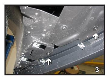
Using a 5.5MM socket, remove two bolts that are located underneath. Set bolts aside to be reinstalled later. Do this on both sides of the vehicle.
