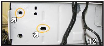
12. Using a 1 1/4" hole saw, drill two 1 1/4" holes into the frame, so an extension can be used to tighten up bolts. Do this to both sides of the vehicle.
