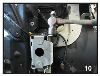
10. You will need to hit the top of the frame a couple times with a hammer to get it level. You can use a straight edge as a guide. Do this to both sides of the vehicle.
