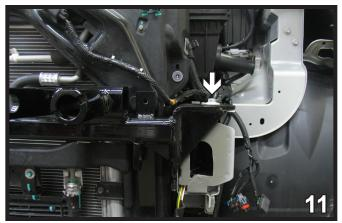
11. Place baseplate on top of frame and line up the holes in the baseplate with the existing holes on top of the frame. Insert one existing 13MM bolt removed in step 7, to hold baseplate into place. Do this to both sides of the vehicle. Use a floor jack to hold the radiator up in place.
