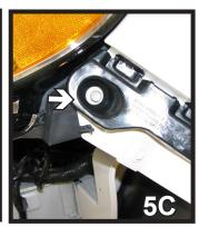
Using a 10MM socket, remove four bolts from the headlight assembly. Remove headlight by pulling
