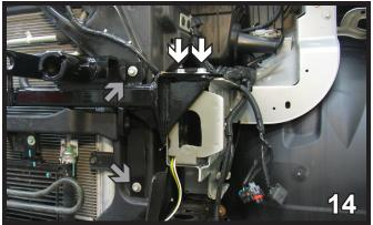
14. After the bolts in Step 13 are installed, you can reinstall the top two 13MM bolts (white arrows) removed in Step 7 and also the two 10MM bolts (gray arrows) removed in Step 7 to hold the radiator support back in place. Do this to both sides of the vehicle. (See note on Step 7.)
