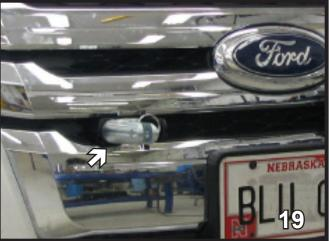
19. Align the fascia to its original position and using a utility knife, trim grille area in front of the attachment tabs. This will then create an opening for the tabs to come through, when reinstalling the fascia. Do this to both sides of the vehicle.
