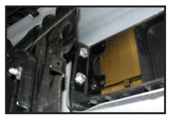
10. Install the electrical bracket on either side of the vehicle depending on the location of the plug in of the coach. Hold up the bracket and mark on the back side. Attach with 1/4"-20 x 3/4" hex bolts, 1/4" lock washers, 1/4" flat washers and 1/4"-20 whiz nuts
