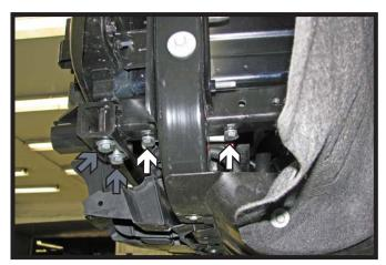
9. Models equipped with tow hooks: Slide the baseplate into position on the frame. Install two (2) 10MM-1.5 x 80MM bolts with 10MM lock washers into the bottom holes (white). Install 10MM-1.5 x 100MM bolts with 10MM lock and 3/8" flat washers thru the baseplate into the bumper on both the front holes (gray). Tighten all hardware. Do this on both sides of the vehicle.
