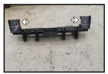
12. Trim the plastic support on the backside of the fascia as shown for baseplate clearance.
