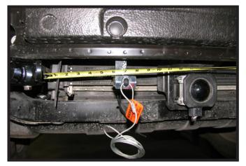
Optional Breakaway: In the desired location, install the bracket to the bumper with a #10-16 x 1" self drilling screw. Attach the breakaway to the bracket with a 1/4"-20 x 3/4" bolt and 1/4"-20 lock nut.
