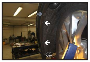
In the wheel well, using a 10MM socket, remove the top screw (gray). Using a 8MM socket, remove the lower screw (black). Then remove the two (2) plastic rivets (white). Do this on both sides of the vehicle.
