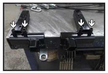
Prior to installing the baseplate to the vehicle, install the appropriate spacer tubes into the slots of the baseplate. The tubes will vary depending on whether the vehicle is equipped with tow hooks or not. Reference page 3.
