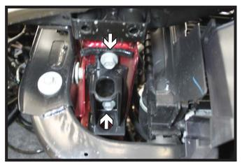
8. **Models equipped with tow hooks:** Using a 16MM socket, remove the two (2) bolts from the tow hook bracket. Remove the tow hook bracket from the vehicle. Do this on both sides of the vehicle.
