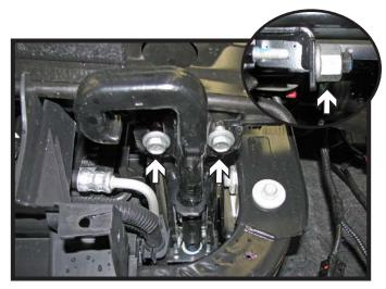
7. **Models equipped with tow hooks:** Using a 16MM socket, remove the two (2) bolts from the front side. Then using a 30MM socket or wrench, remove the nut from the backside of the tow hook. Remove the tow hook from the vehicle. Do this on both sides of the vehicle.
