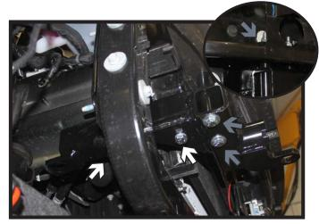
10. **Models equipped without tow hooks:** Slide the baseplate into position on the frame. Install two (2) 10MM-1.5 x 80MM bolts with 10MM lock washers into the bottom holes (white). Insert 3/8"-16 x 4-1/2" bolts with 3/8" lock and flat washers into the front holes with the locking plate and 3/8"-16 lock nuts on top of bumper (inset). Tighten all hardware. Do this on both sides of the vehicle.
