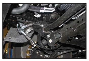
11. Attach the permanent baseplate safety cables to the provided convenience link on the baseplate. The photo shows the recommended installation of the cables to frame of vehicle. Additional options may interfere with suggested mounting; in this case, secure the cables to a solid piece of the frame as described in the General Information sheet. Be sure the safety cables do not rub against any hoses or moving parts. Do this on **BOTH** sides of the vehicle.
