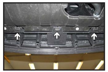
3. On the underside of the fascia, turn the three (3) locking knobs 90° to release.
