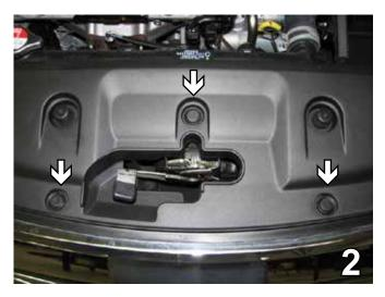
2. Remove three push pins from the middle in order to remove the radiator cover. Set cover and push pins aside to be reinstalled later.
