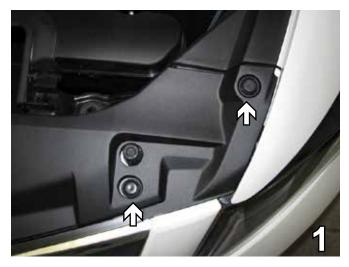
1. Remove two push pins from the side in order to remove the radiator cover. Do this to both sides of the vehicle. Set push pins aside to be reinstalled later.
