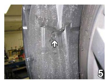
5. On the driver's side, remove the push pin just forward of the front tire in the wheel well. Set the push pin aside to be reinstalled later.
