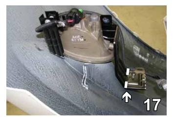
17. On the passenger side, trim the fog light bracket along the bend.
