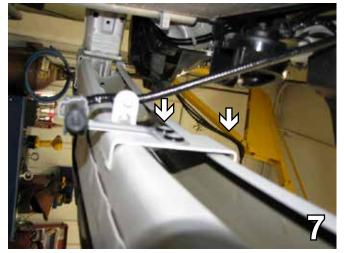
7. Behind the bumper, disconnect the temperature sensor by removing two push pins before taking the bumper off.
