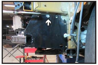
11. Drill one (1) 3/8" hole and install 3/8" bolt with nylon lock nut, tighten fully. Do this on both sides of the baseplate. Ensure baseplate is level.
