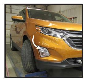
5. Pull the corners of the fascia away from the vehicle. Disconnect all electrical connections and pull the fascia from the vehicle. Set aside to be reinstalled later.
