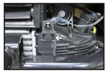
15. Drill a 1/4" hole in temperature sensor holder and reinstall on the grill using existing push pin. Reinstall temperature sensor.
