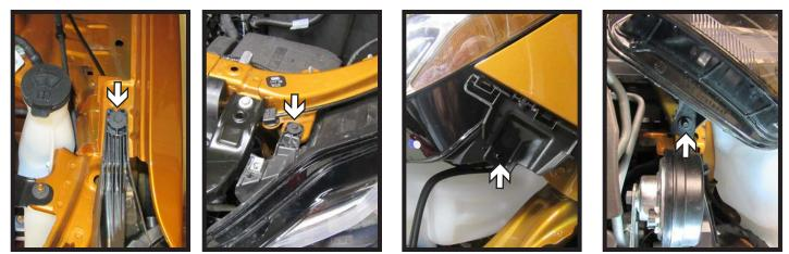
6. Using a 7MM socket remove the four (4) bolts attaching the driver side head light. Remove and set aside to be reinstalled later.
