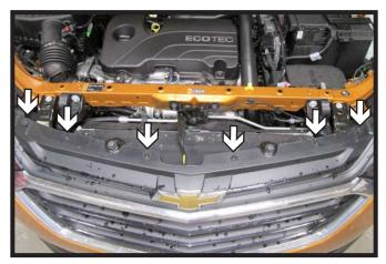
Using a T15 Torx, remove the six (6) screws from the top edge of the fascia. There are three (3) on each side.
