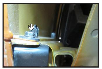
3. Using a 7MM socket, remove the bolt from inside the wheel well. Do this for both sides of the vehicle.
