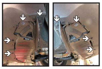
4. Using a 7MM socket, remove the eight (8) bolts from the underside of the fascia, four (4) on each side.
