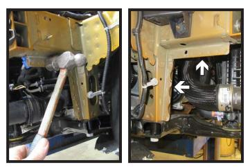
9. Use a hammer to tap the metal frame pieces inward slightly, about 1/8", to allow clearance for baseplate. Do this on both sides of the vehicle.
