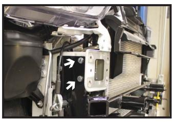
10. Using a 3/8" drill bit, drill the remaining holes thru the frame. Install the 3/8" hardware and fully tighten. Do this on both sides of the vehicle.
