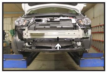
12. **Optional Breakaway:** Using a self tapping screw, attach the bracket to the lip of the bumper in the desired location. Attache the breakaway to the bracket with the supplied 1/4" hardware.
