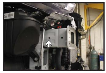
8. Using a 3/8" drill bit, ream out the existing rear passenger side hole.
