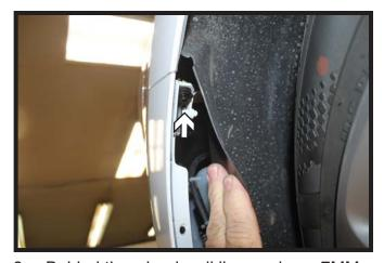
Behind the wheel well liner, using a 7MM socket, remove the screw from the fascia/ fender joint. Do this on both sides of the vehicle.
