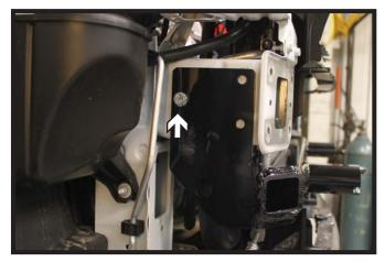
9. Align the baseplate to the frame, installing the 3/8" hardware into the rear holes on both sides. Level the baseplate and fully tighten the hardware.
