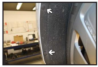
2. Remove the two (2) push pins from along the edge of the wheel well. Do this on both sides of the vehicle.
