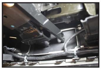
10. Partially reinstall the fascia again. On the inside of the frame, hold the convenience link against the frame and fascia an mark the area to trim. Do this on both sides of the vehicle. Remove the fascia and trim.
