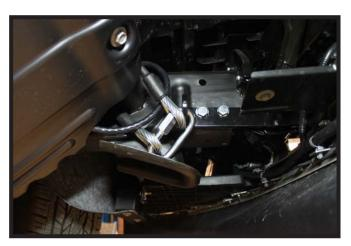
12. Attach the permanent baseplate safety cables to the provided convenience link on the baseplate. The photo above shows the recommended installation of the cables to frame of vehicle. Additional options may interfere with suggested mounting; in this case, secure the cables to a solid piece of the frame as described in the General Information sheet. Be sure the safety cables do not rub against any hoses or moving parts. Do this on **BOTH** sides of the vehicle.
