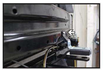
14. **Optional Breakaway:** Attach the bracket to the metal bumper with the #10-16 x 1" self drilling screw at the desired location. Attach the breakaway to the bracket with the 1/4" hardware provided.
