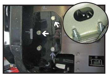
10. Drill out remaining holes with a 13/32" drill bit. Insert a 3/8"-16 x 1" hex bolt, 3/8" lock washer and 3/8"-16 hex nut in the other bottom hole (gray). In the top two (2) holes (white), install 3/8"-16 x 1-1/2" hex bolts and 3/8" lock washers attached to 3/8"-16 nut plates inserted up inside the bottom of the frame. Do this to both sides of the vehicle.
