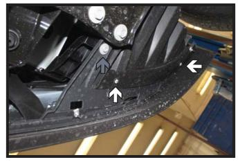
4. On the underside of the fascia, using a T20 Torx, remove the outer screws (white). Then using a 10MM socket, remove the inner screw (gray). Do this on both sides of the vehicle. Disconnect all electrical wiring and remove the fascia from the vehicle.
