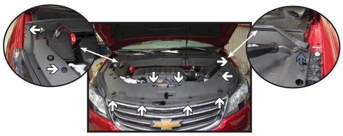
Remove the ten (10) push pins from the top edge of the fascia shroud (white). Then pry up the ends of the rubber strip on each side, releasing the clip underneath (gray). Remove the shroud from the vehicle.
