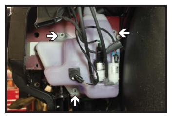
5. On the driver side, using a 10MM socket, remove the three (3) nuts from the washer fliud reservoir. Disconnect all lines and electrical connections, then set reservoir aside.
