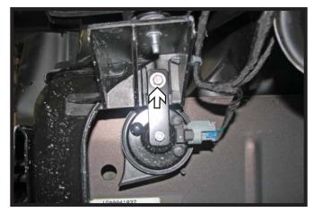
Using a 10MM socket, remove the screw from the horn bracket and set horn aside. Do this on both sides of the vehicle.
