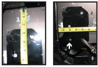
9. Tip the baseplate onto the frame. Measure down 2-13/16" from the top of the frame to the top of the baseplate. Measure 6-1/4" from the front of the frame to the back of the baseplate. Level the baseplate and clamp into position. Using the baseplate as a template, drill a 13/32" hole (white) and insert a 3/8"-16 x 1" hex bolt, 3/8" lock washer and 3/8"-16 hex nut. Do this to both sides of the vehicle. Tighten down fasteners.
