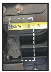
Using a reciprocating saw, trim an area on the frame approximately as shown. Cut the bottom flush with the bottom rail (gray) and vertically just inside the rib (approximately 1-5/8") then 2-1/2" back at the top. Do this on both sides of the vehicle.
