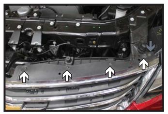
Using a T20 Torx, remove the seven (7) screws from the top edge of the fascia (white). There are four (4) on the driver side and three (3) on the passenger side. Using a 7MM socket, remove the two (2) screws from the top edge of the fascia corners (gray). There is one (1) on each side of the vehicle.
