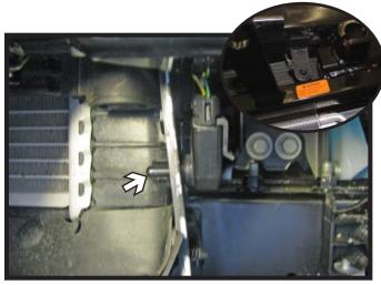
Reinstall the temperature sensor to its original location or on the driver's side, using a 1/2" drill bit, drill a hole into the plastic shrouding. Then snap the temperature control into the hole.
