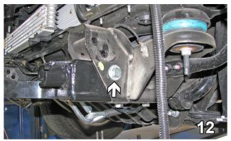
12. Insert 1/2-13 x 1 1/4" hex bolts with 1/2" lock washers into both sides of the base plate. Be sure to use Loctite red on all bolts. Do this on both sides of the vehicle.
