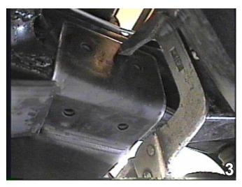
Clamp the passenger's side with the large vise grips. Using the baseplate as a template, drill four (4) holes using the 13/32" drill bit.
