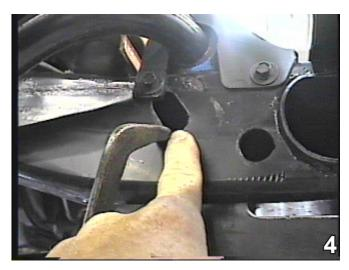
4. Using the 3/8"-16 x 1-1/2" hex bolts, 3/8" lock washers, and the 3/8"-16 nut plates, insert the nutplate into the frame and align with the holes. Tighten ALL bolts.
