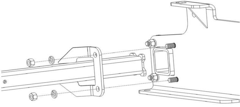
2. If there was not at least 1/4" of threads sticking passed the nuts before they were removed, the rib neck bolts will need to be replaced. One at a time, Replace the two Front **Rib Neck Bolt** on the Super Hitch Cross Tube with the provided 1/2"-13 x 1-7/8" **Grade 8 Ribbed Neck Bolts**
