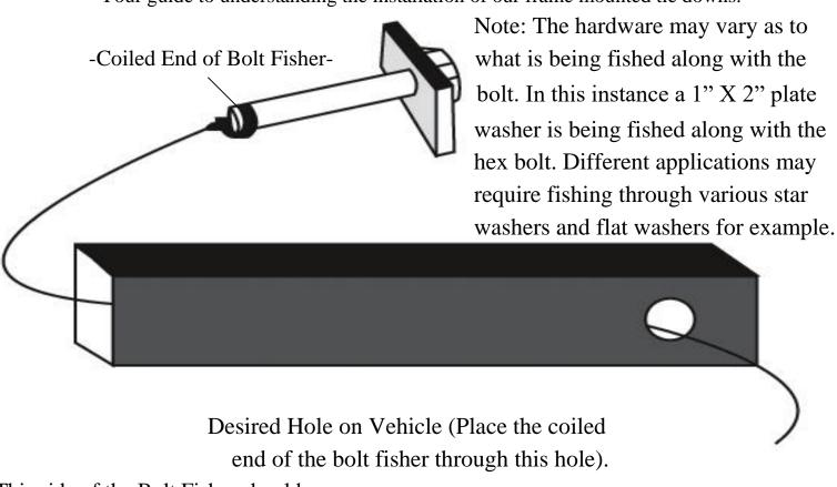
This side of the Bolt Fisher should come out of a hole where the required hardware (for example 1" X 2" plate washer) can pass
