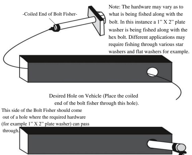
This bottom example shows the bolt when it's completely fished through the vehicle. You may find it easier to keep the bolt fisher attached until you get the tie down receiver in place so that the bolt doesn't fall into the vehicle frame.
