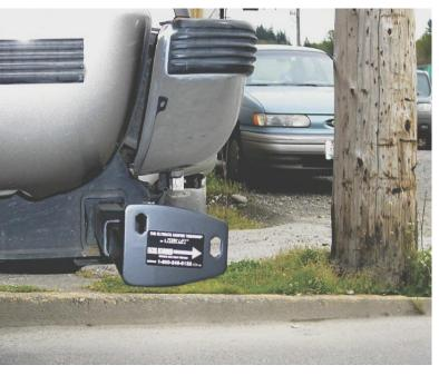
IMPORTANT NOTE: Your tie down inserts are designed to have clearance inside of the receiver. This is to account for road debris, as well as aid in installation and removal. Some rattle may be expected if the inserts are left installed while not under load from the camper.
