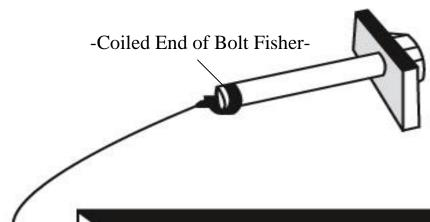
Note: The hardware may vary as to what is being fished along with the bolt. In this instance a 1" X 2" plate washer is being fished along with the hex bolt. Different applications may require fishing through various star washers and flat washers for example.
