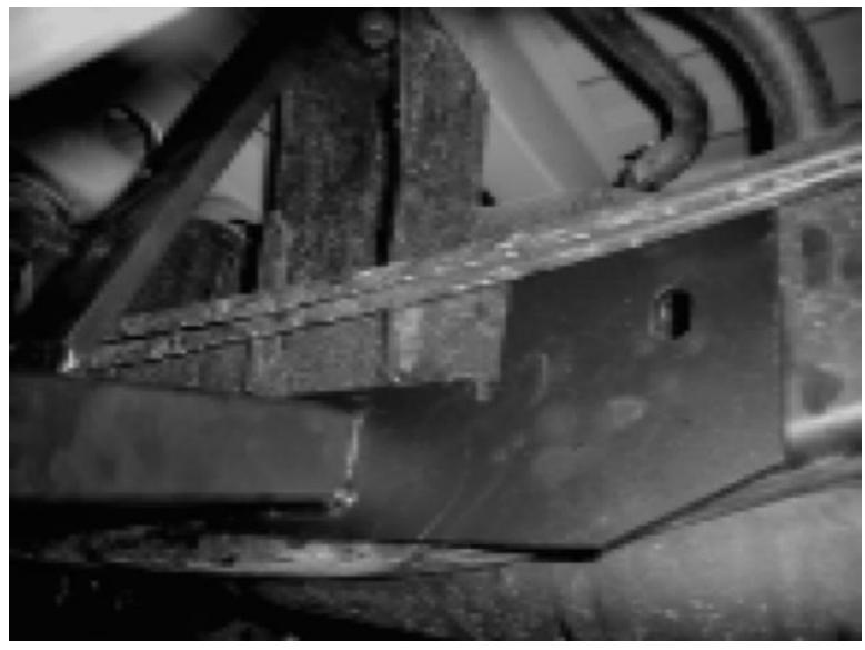
**NOTE:** *The bolt and plate washer must be put into the frame separately*
