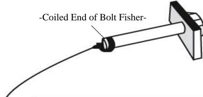
Note: The hardware may vary as to what is being fished along with the bolt. In this instance a 1" X 2" plate washer is being fished along with the hex bolt. Different applications may require fishing through various star washers and flat washers for example.
