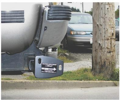
*IMPORTANT NOTE:* Your tie down inserts are designed to have clearance inside of the receiver. This is to account for road debris, as well as aid in installation and removal. Some rattle may be expected if the inserts are left installed while not under load from the camper.
