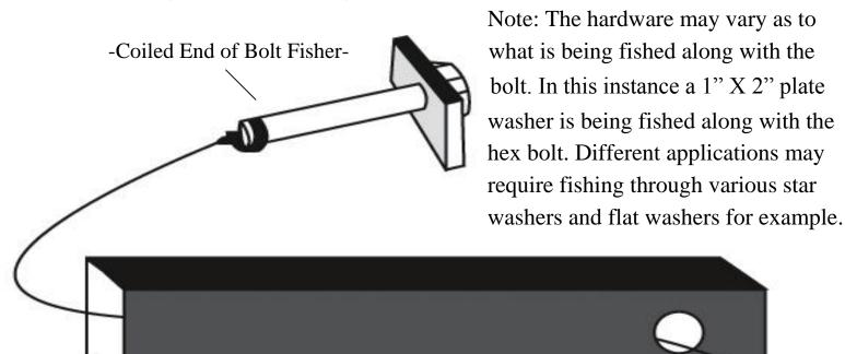
Desired Hole on Vehicle (Place the coiled end of the bolt fisher through this hole).
