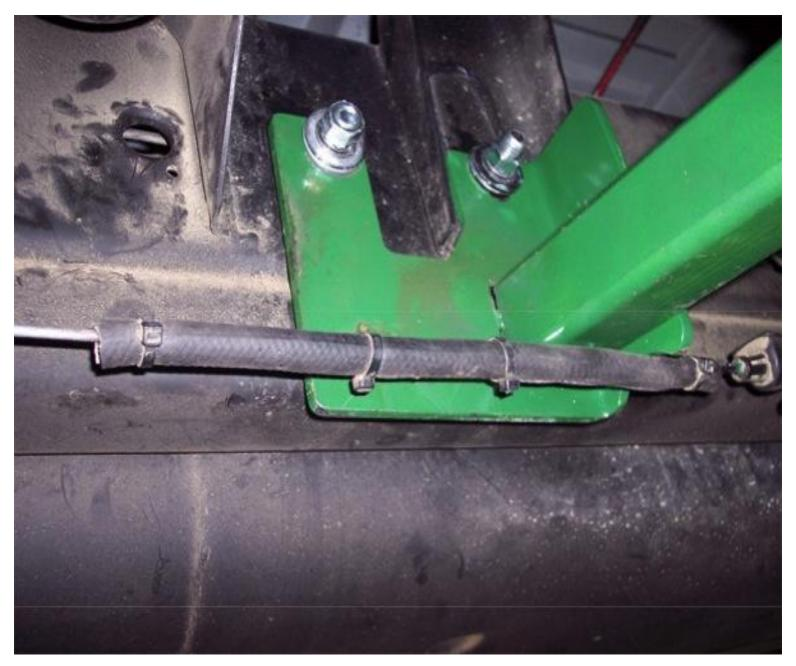
Depending on the year of your vehicle, the emergency brake line will be positioned either above or below the tie down receiver. To prevent any possible emergency brake line damage, we have provided you with a 3/8" piece of tubing to wrap around the line and four tie straps to secure the tubing. You will have to slit the tubing lengthwise in order to slip the line inside prior to securing the tie straps as shown above.
