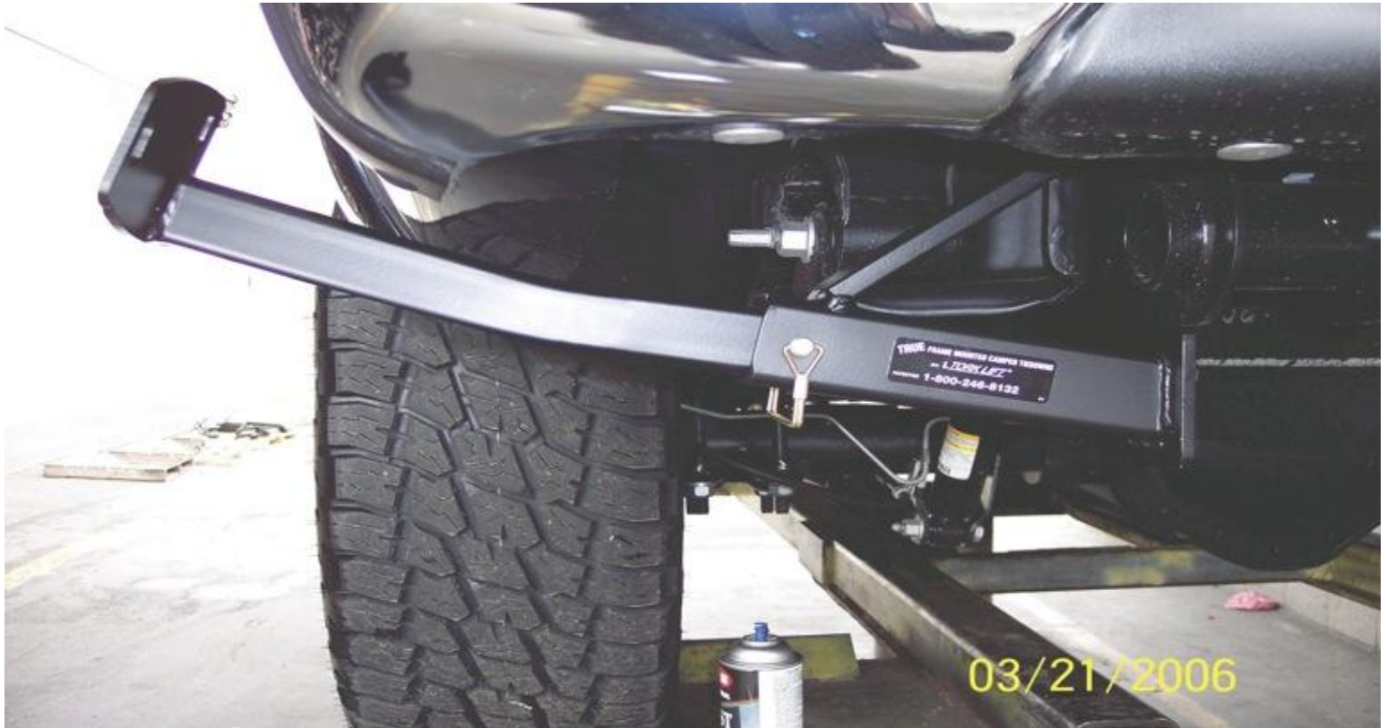
Correct insert installation C3205 ONLY
