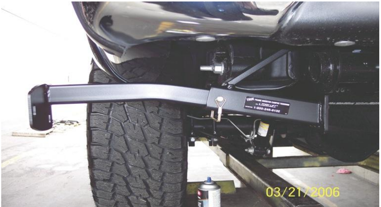
Correct insert installation C3205 ONLY
