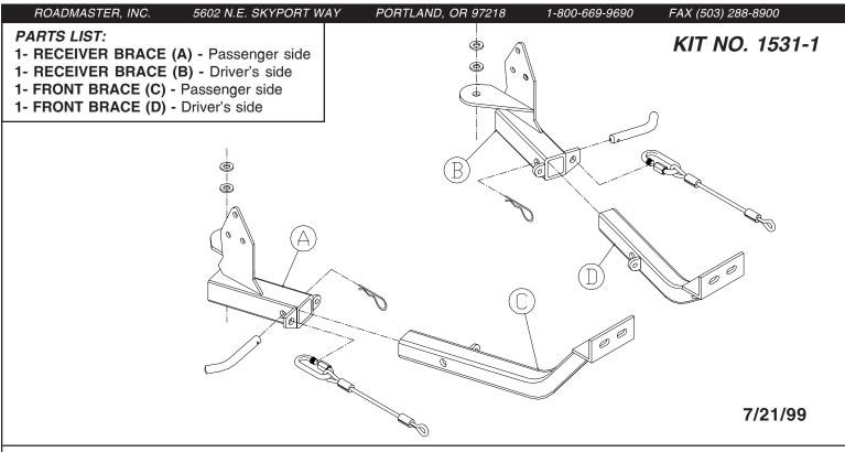
*IMPORTANT:* All brackets *must* be assembled with all the bolts left loose for final adjustment & positioning (before tightening) unless otherwise instructed. All bolts *must* be torqued for proper strength. If more than one bolt is used per fastening point, the diagram may only show one.
