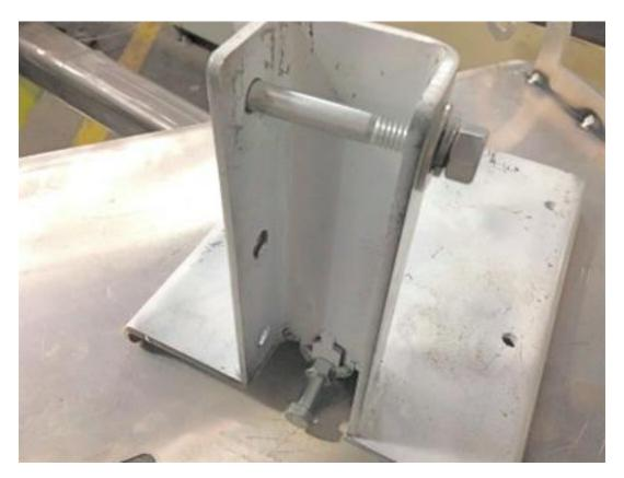
STEP 3- Follow the step associated with your part number. Install the U-COLLAR onto the extension at this time.
