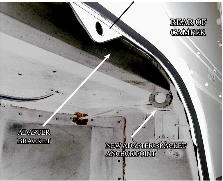
**NOTE:** Depending on your installation, using the supplied Rectangular Shim 2-1/2 " X 1-1/4 " X 1/2 " may be required for use on the over sized holes on the camper anchors.
