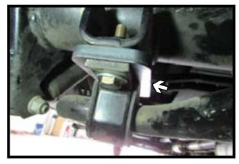
2. If the vehicle has a sway bar equipped, install the sway bar spacers shown in the right photo prior to installing the axle bracket.
