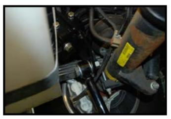
3. Position the frame bracket onto the driver side frame rail and loosely secure it with the nut plate frame bracket and the 5/8" hardware. Loosely install the 1/2"-20 bolts and jam nuts into the frame bracket.
