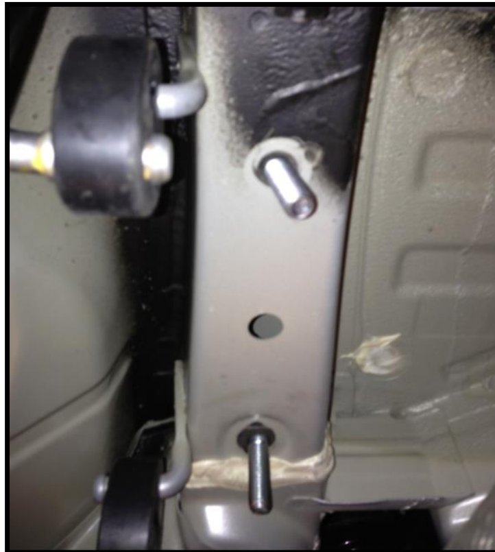
Figure (4.2) shows a successfully fished bolt with the 1/2"x2" bolt head resting on top of the 1/2" internal tooth star lock washer and plate washer, through the frame rail holes.
