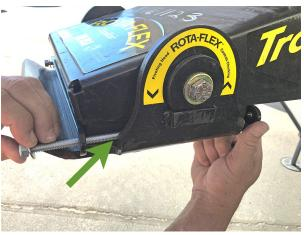
4. Now place the remaining washers and lock nuts onto the ends of the threaded bolts as shown right.
