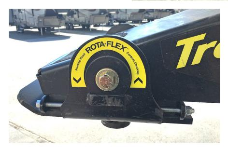
5. Finally, tighten the lock nuts down. Be careful not to over tighten and strip them - they simply need to keep the two bars in place.
