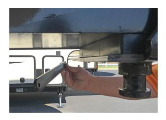
2. Place the other steel bar in the back of the pin box above the lip as shown left and below.
