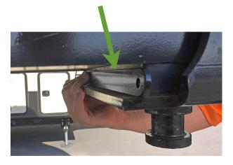
3. Next push the two threaded bolts (with washers in place) through holes in the steel bars. Make sure both bolts are inside of the rotating plate as shown right (arrow).
