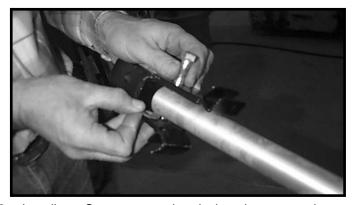
2. Install new Sentry connecting clevis, using new washers, 1/2" bolts, and locknuts. **Note:** Excali-bar, and Aluminator use gray (thick) washers inside of clevis. Kwik-Tow uses white (thin) washers. Tighten 1/2" bolt so that there is a slight drag when pivoting clevis side to side. **Note:** On Kwik-Tow, long leg of clevis goes on top side of tube.
