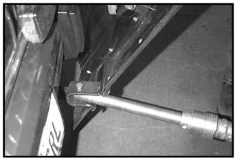
4. Slide right and left wings into Sentry connecting clevis until wings are approximately 1/4" away from bottoming out against clevis.
