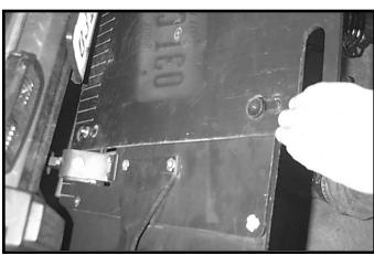
**5.** Slide one side of center section on left wing and the other center on the right wing and push down to latch in key slots.
