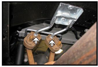
4. Further back, drop the exhaust by sliding the rubber insulators off the hanger studs. Note: Using silicone spray on the insulators eases removal from hangers.
