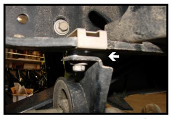
12. Reinstall the exhaust hanger to the frame with three (3) 3/8" washers in between the frame and hanger. Reinstall the exhaust to the factory hangers. Reinstall the spare tire per the vehicles owners manual.
