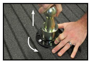
1. Rotate the locking collar to release the latch pawl. Pull straight up on the ball to remove from the hitch.
