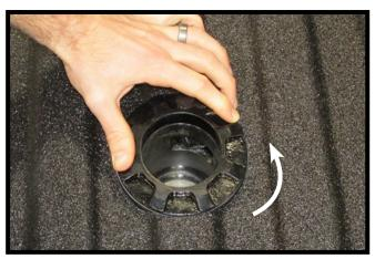
10. Check the rotation of the top collar at this time to insure the bed is not rubbing against it and it can rotate freely. If necessary drop the center section and remove any obstructions.
