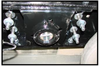
11. Fully tighten all cross member/center section hardware. Then using a 19/32" drill bit, drill the two (2) holes closest to the ball thru the bed. Do this on both sides. Insert the 1/2"-13 u-bolts thru the holes from the topside. Install a 1/2" flat washer, spring, another 1/2" flat washer and 1/2"-13 lock nut onto each u-bolt stud. Tighten until the washers are touching the spring without compressing it.
