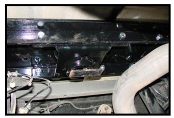
7. On both sides of the center section, bolt the cross members to the center section with four (4) 1/2"-13 x 1-1/2" bolts with 1/2" washers and 1/2"-13 lock nuts on the inside. Do not fully tighten hardware.
