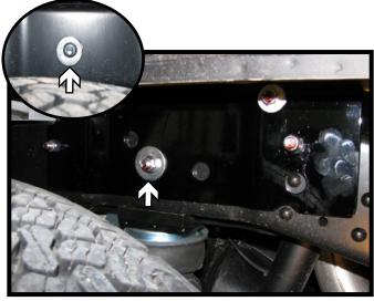
9. Repeat the same steps from step #8 on the passenger side. If the vehicle is equipped with air bags, the nut and washer must be removed prior to support plate installment (inset). Then reattach the washer and nut to the stud after the support plate is installed. Fully tighten both support plates hardware.
