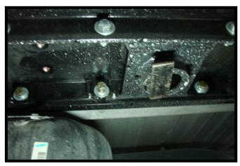
8. Install the center section in between the cross-members and up through the 5" hole in the truck bed. Insert all bolts into the cross-members and center section.
