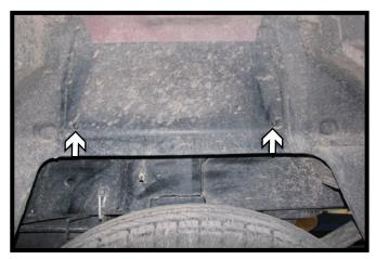
4. Using a Phillips screwdriver, remove the two (2) screws on the wheel well cover just above the rear tires. Do this to both sides of the vehicle. Set the covers aside to be reinstalled later.
