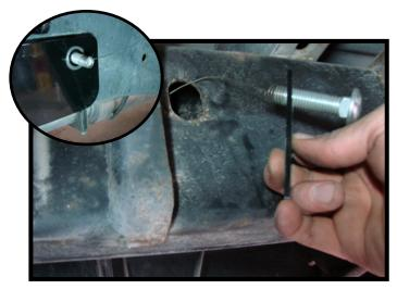
12. Insert the fishwire through the side plate and into the vehicle frame. Retrieve the fishwire through the access hole on the inside of the frame and install a plate and carriage bolt. Pull the plate and carriage bolt through the frame and out through the side plate.
