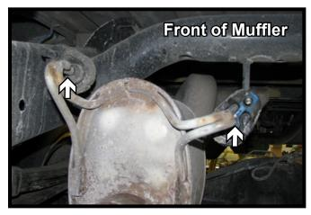
Drop the exhaust by sliding the three (3) hangers out of the rubber insulators. There is one
