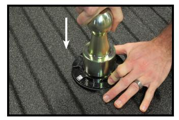
Align the ball with the collar and drop the ball into the hitch. Release the locking collar.
