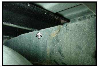
7. Slide the front cross-member into position across the top of the frame as shown. Install the rear cross-member in a similar manner across the frame and push up against the bed rail until center section installation (reference photo in step #6).
