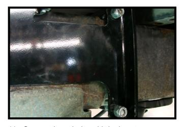
11. Secure the u-bolts with lock-nuts.
