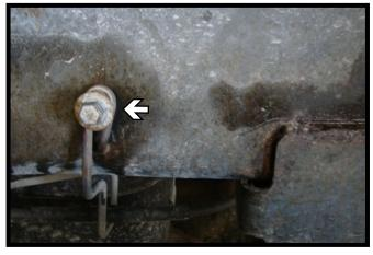
On the driver side only, remove the emergency brake bracket bolt and set aside.
