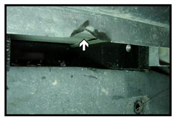
6. On passenger side, locate the hole in the bottom rib of the truck box just above the frame. Insert the rear angle cross-member through the opening between the top of the frame and the box directly above the hole and lift to create a crease in the rib to allow room to install the cross-member across the top of the frame.
