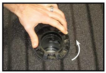
Rotate the locking collar to release the latch pawl.
