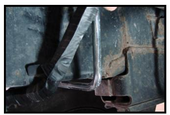
10. Install each u-bolt around the frame and through the holes in both side plates. On the drivers side, pull back the wiring loom and install the u-bolt directly against the frame. Be sure not to pinch any wiring.
