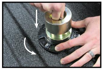
Rotate the locking collar to release the latch pawl. Align the ball with the collar and drop the ball into the hitch.
