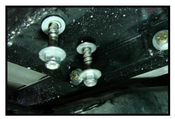
14. Using a 19/32" drill bit, drill the two (2) u-bolt holes thru the bed. Do this on both sides of the center section.
