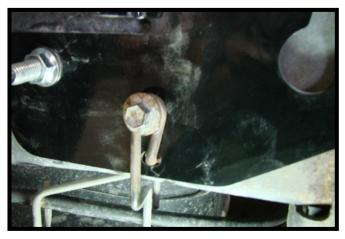
Reinstall emergency brake line bracket using the existing bolt through the two hole in the side plate.
