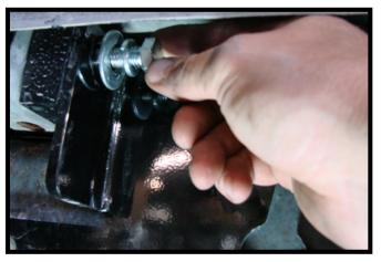
9. Install both side plates and insert corresponding hardware.
