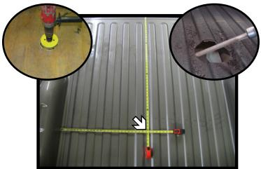
2. On the inside of the bed, measure from the rear (not the tailgate) forward 46-3/16" for a 8' bed or 44-3/16" for a 6'-4" bed and mark. Measure between the wheel wells and mark center. Using a 5" hole saw, drill a hole thru the bed.
