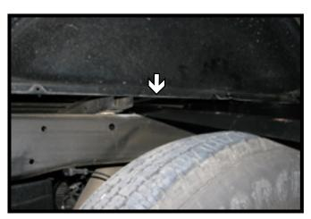
5. Slide the cross members in from the side. Push the flat end in just ahead of the rib. Slide the angle in part way, lift up and bend the rib then finish pushing it in, then bend the rib back. Turn so that the holes are on the lower side, facing down and to the back.
