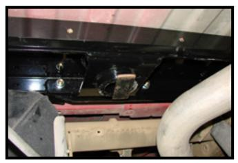
On both sides of the center section, bolt the cross members to the center section with the supplied 1/2" hardware. Do not fully tighten hardware.
