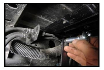
10. Install the fishwire into the hole in the side plate thru the frame and out he nearest frame hole. Install the plate & carriage bolt onto the fishwire and pull thru the frame and out the side plate hole. Install the nut onto the bolt. Do this to both side plate holes on both sides of the vehicle.
