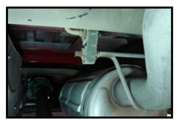
14. Reinstall the exhaust to the factory hangers. Reinstall the spare tire per the vehicles owners manual.
