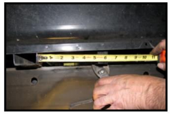
8. On the backside of the bed rib, measure to the 1"x2" cross member. Set to an equal distance on both sides so the hitch is square with the vehicle.
