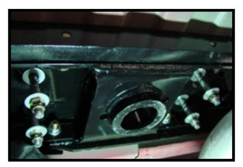
Insert the 1/2"-13 u-bolts thru the holes from the topside. Install a 1/2" flat washer, a spring, another 1/2" flat washer and 1/2"-13 lock nut onto each u-bolt stud. Tighten until the washers are touching the spring without compressing it.
