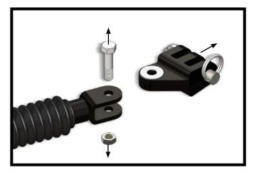
1. Using a 3/4" socket and wrench, remove the existing 1/2"-13 bolt and 1/2"-13 jam nut from the tow bar leg. Remove the existing lug and washers from the tow bar leg. Do this on both tow bar legs.
