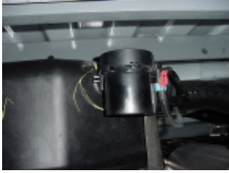
Step 1: Locate the fuel valve.
