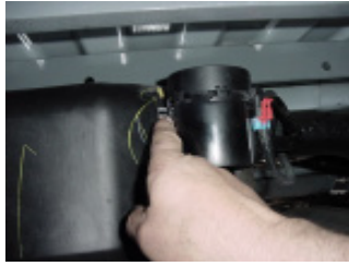
Step 2: Disengage the locking pin.
