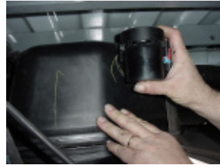
Step 3: Slide fuel valve from bracket.
