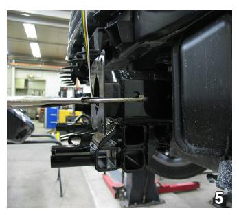
5. Lift baseplate straight up and slide forward up to dimple in frame. Baseplate should be straight and clamped into place with vise grips.
