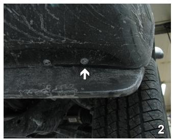
Using a 10MM socket, remove one metric bolt from the front of the fascia. Set bolt aside to be reinstalled later. Do this to both sides of the vehicle.
