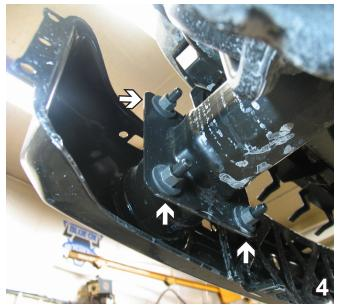
4. Using a 18MM socket, remove three metric nuts from the metal bumper. Set bumper and nuts aside to be reinstalled later. Do this to both sides of the vehicle. Some models may have a tow hook that will need to be removed, if applicable.
