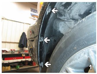
Using a 10MM socket, remove three metric bolts just forward the front tire, on the wheel well. Once bolts are removed from the wheel well, pull plastic back and remove two metric bolts with a 10MM socket. Set bolts aside to be reinstalled later. Do this to both sides of the vehicle.
