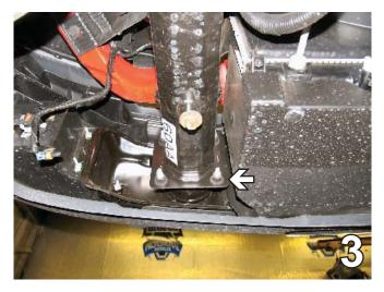
3. Using the 18MM socket, remove four metric nuts. Located just behind the metal bumper, on the frame end. Set the metric nuts aside to be reinstalled later. Pull the metal bumper forward, unplug the electrical connections and set the metal bumper aside to be reinstalled later.
