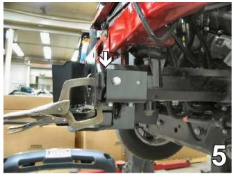
Slide the baseplate onto the frame rail to align 5. forward side hole with existing hole in the frame and clamp in place with the vise grips. Do this to both sides of the vehicle. Insert the nutplate into the end of the frame rail to align with the existing hole, tighten the 1/2-13 x 1 1/2" hex bolt and lock washer with the 3/4" socket. Do this to both sides of the vehicle.
