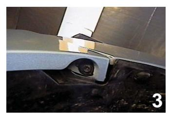
Remove two bolts from the underside of fascia's edge, just forward of the front tire. Do this on both sides of the vehicle. Disconnect electrical appliances, pull fascia forward to remove, and set aside to be reinstalled later.
