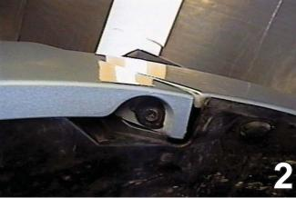
Use the 8MM socket to remove a bolt from inside the front wheel well on fascia's corner, just forward of the front tire. Set the bolts aside to be reinstalled later. Do this to both sides of the vehicle.
