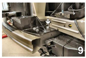
9. Slide bumper between frame and baseplate to align with existing mount locations. Place (2) 3/8" flat washers between the baseplate and the top of the metal bumper. Insert two 8MM-1.25 x 30MM hex bolts with 5/16" lock washers and 5/16" flat washers and tighten. Tighten the bolt near the back of the baseplate, as indicated by the white arrow in the photo above. Do this to both sides of the vehicle.
