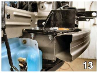
13. Place the backing plate on the bottom side of the frame webbing to align with drilled holes, insert the 3/8-16 x 1 1/2" hex bolts and 3/8" flat washer into this hole, tighten the 3/8-16 hex nut and 3/8" lock washers.
